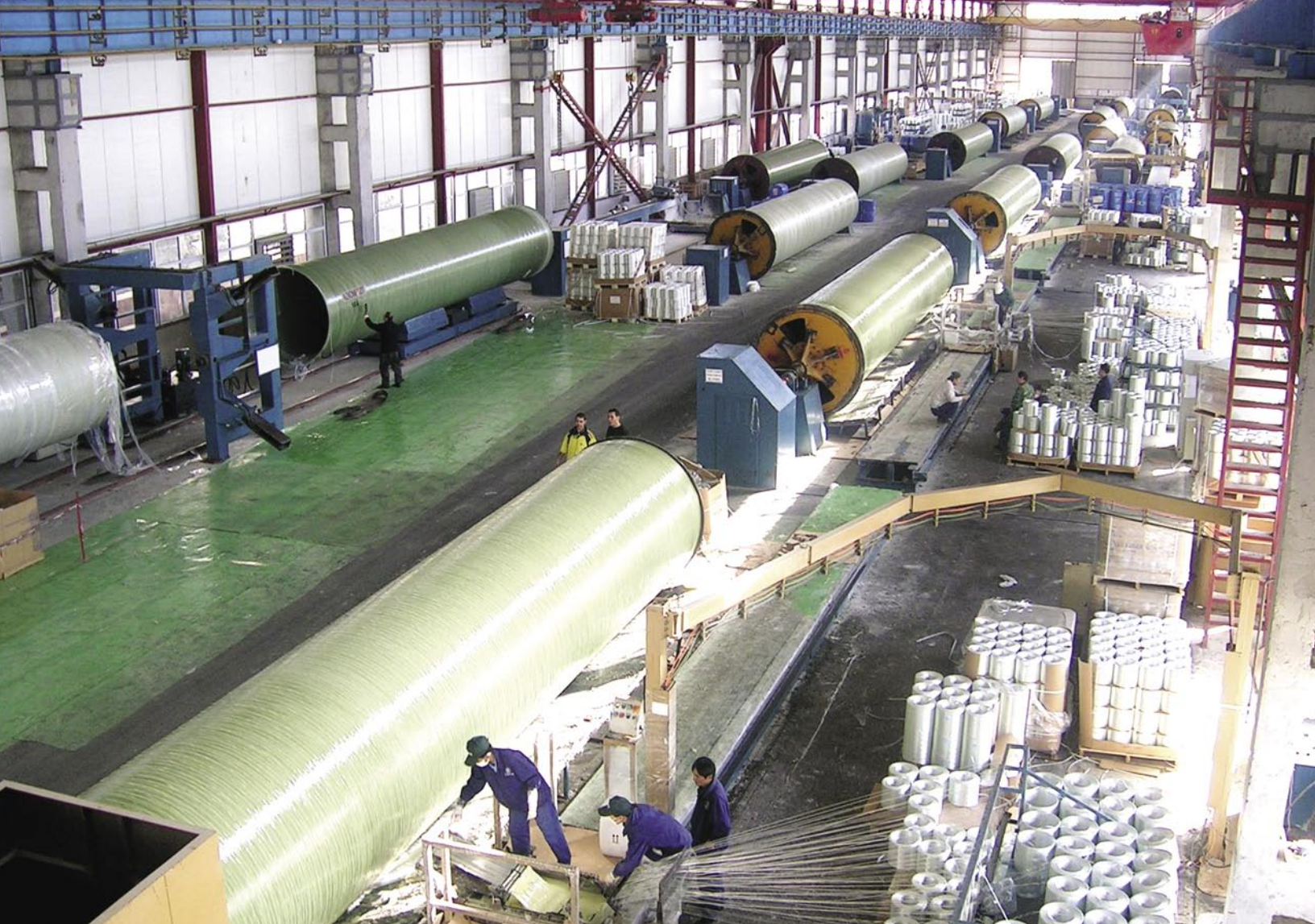
The Azkompozit factory has 15 computerised filament winders.
